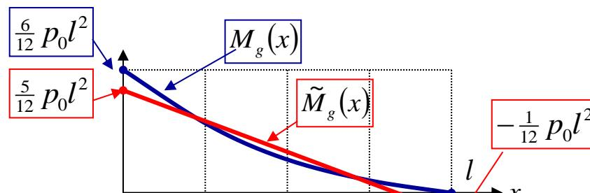
**Example:** cantilever beam loaded with a uniformly distributed transverse loading and point loads
